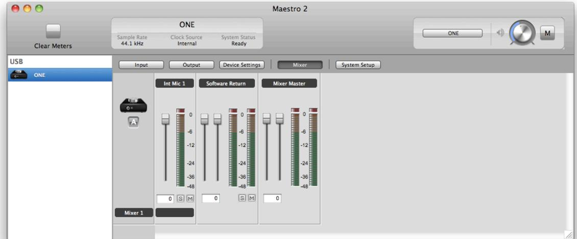
On the Output tab of Maestro, set the output to Mixer.
