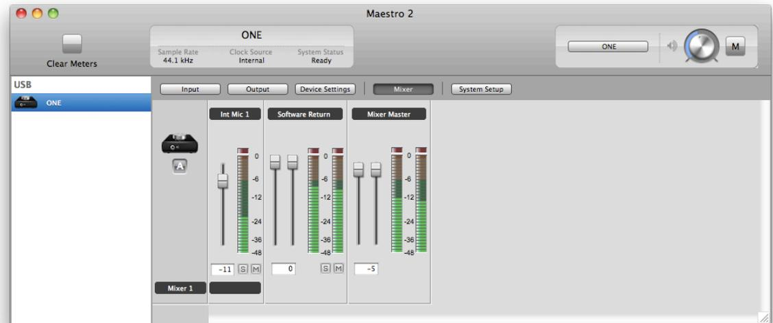
Now start playback in your recording software. The playback signal should be displayed on the Software Return and Mixer Master's meters. Use the Software Return and Input faders to establish your desired balance between the input and playback signals. If you've found a good balance but the Mixer Master's Over LEDs light, reduce the Mixer Master fader.
