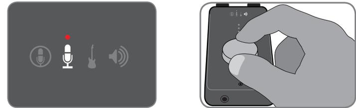
To select another input as the active input, open a software control panel (either Apogee Maestro, Audio MIDI Setup, or the GarageBand/Logic control panel) and select the desired input, as described on the following pages.
